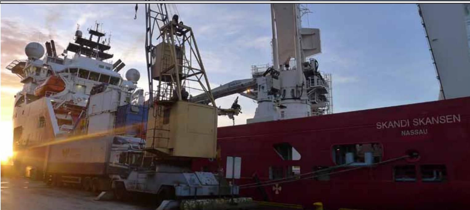
The Skandi Skansen, a versatile multipurpose Construction Anchor Handler docked in Kristiansand before heading to Dundee to commence its next charter. The vessel is 109 meters long with an A-Frame, winch capacity of 500 T and a 250t offshore crane including a working ROV.
