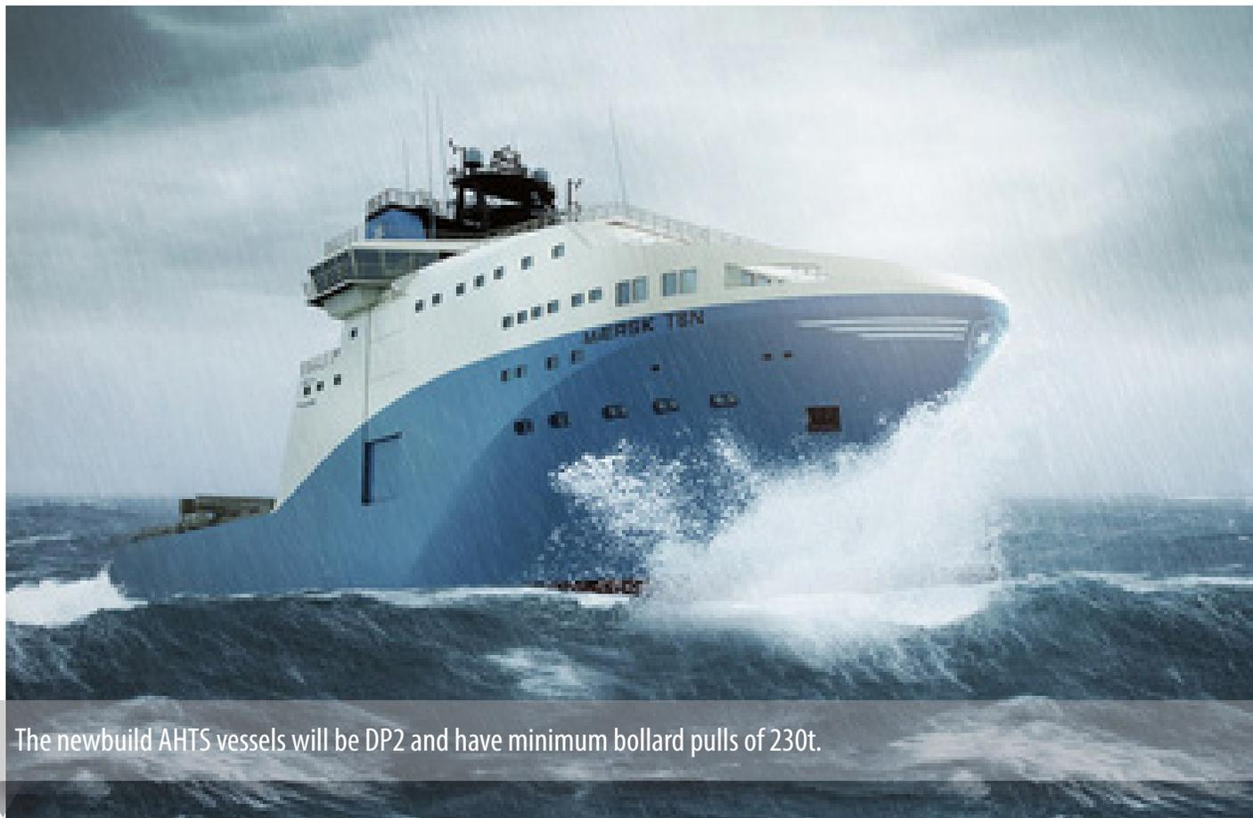
The newbuild AHTS vessels will be DP2 and have minimum bollard pulls of 230t.
