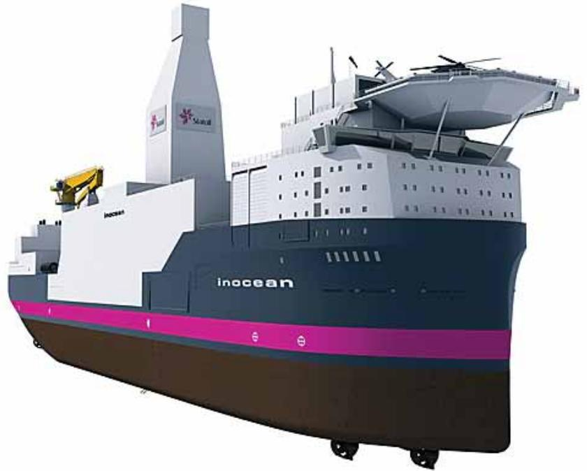
The design concept for the Cat I rig has been given to **Inocean** along with an option on the Front End Engineering Design, with the winning design based on the INO-80 drillship. The rig will have to have a hull able to operate in ice conditions of up to 2 meters and is specially designed for Arctic environment.
